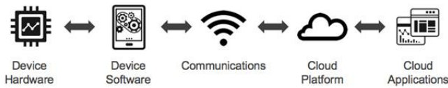
Fig. 1. An example of a commonly used rough model of the IoT technology stack [2].
